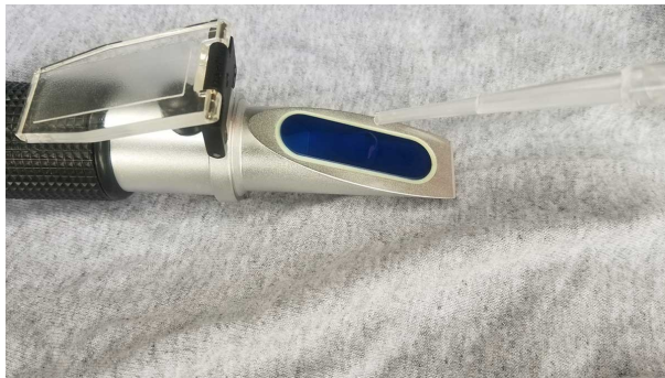
Place a drop or two of fluid on the screen
