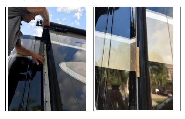
8. With the trim piece open, remove the set screw from the area shown below. The picture shows the top of the slide. The set screw keeps the motor in place.
