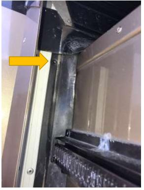
9. Go back into the coach and remove the rubber and plastic stripping that covers the motor wire and hides the motor. You'll need to unplug the motor from the wire here and then pop up the motor and then pull it out.
